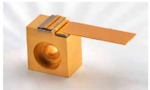
Fig. 6. Diode laser with one individual emitter (C mount)
